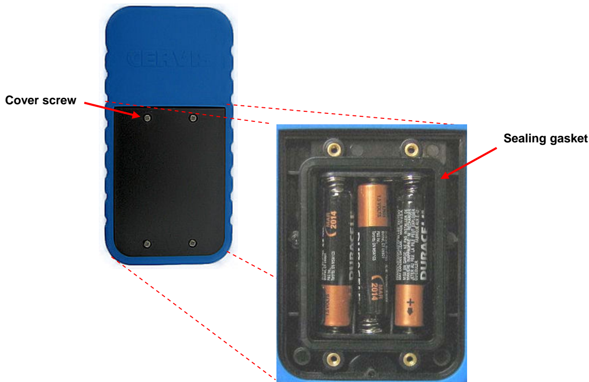
Figure 6. Handheld Battery Installation
