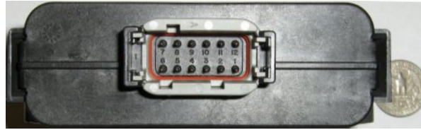
Figure 3. Female Twelve (12) Pin Connector
