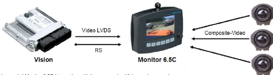
Image 1.4 Monitor 6.5C interaction with its accessories Vision and composite camera
