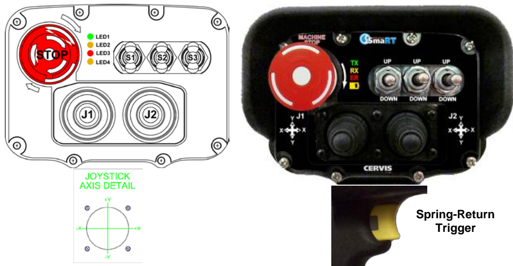
Figure 2. Top Plate Switch and Joystick Layout
