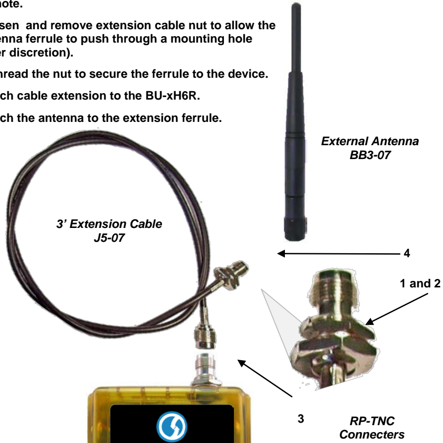
Figure 4. Antenna Extension Kit Installation
