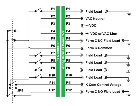
The wiring configuration shown is for a BU-xH1R5 — no CAN connection.
