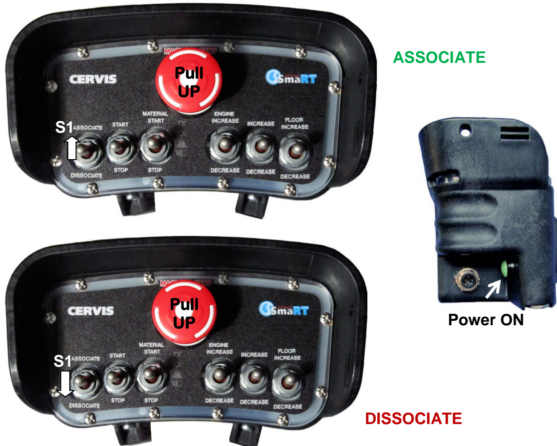
Figure 8. MCB Switch Actuation for Associate and Dissociate
