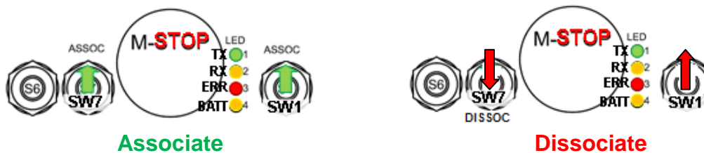
Figure 9. PG Switch Actuation for Associate and Dissociate
