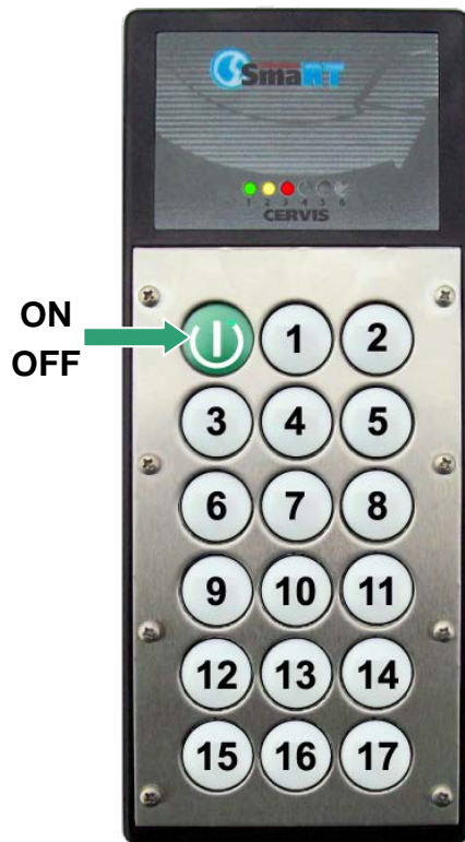
Figure 5. Handheld Buttons and Typical Button to Output/Input Mapping
