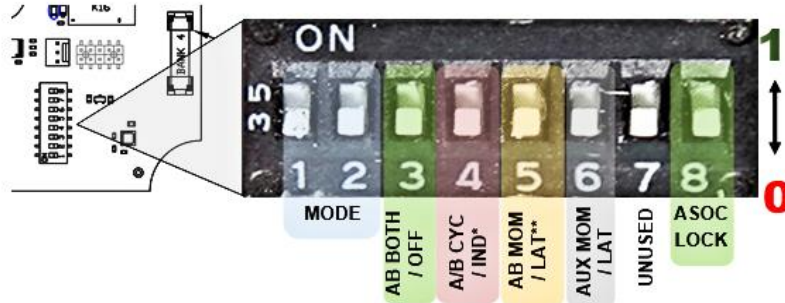
Figure 1. MU-9X15 SW01 DIP Switch Assignments
