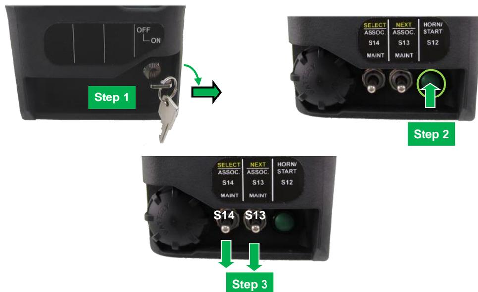
Figure 5. Clearing the ID (Factory Reset)
