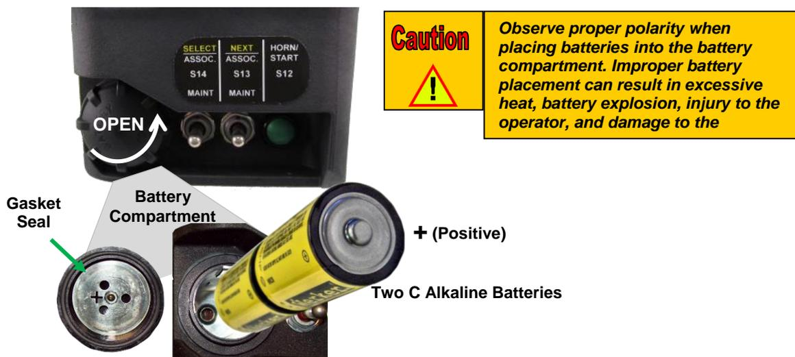
Figure 2. Warrior Console Box Battery Installation
