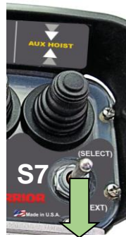
Figure 4. Method 2 Virtual Unlock Switch 7– Push and Hold Down
