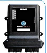
The versatile EBU-xH24XF base units feature an H-Bridge, sixteen FET (field effect transistor) highside switching outputs or switch-to-ground digital inputs, two Form C relays, and CAN Bus control capability.
