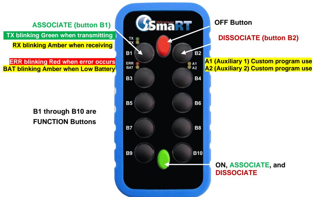
*Figure 6. HH-x10 Front Panel*
