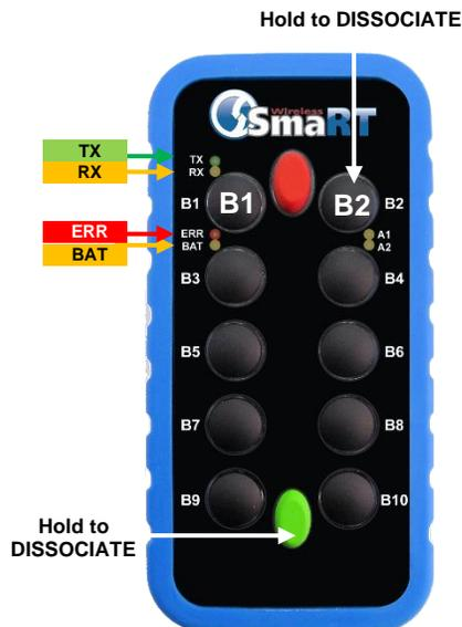
*Figure 4. Dissociate an HH-x10 Remote control from a Base Unit*
