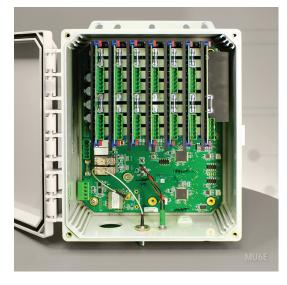
The **MU6E** is a modular receiver intended for use in industrial systems including overhead bridge cranes. The MU6E is self-contained and can be configured with various input/output modules accommodating various I/O requirements. The MU6E will accept control commands from the full range of Cervis Warrior transmitters including the multi-joystick multi-axis Warrior Console Box.
