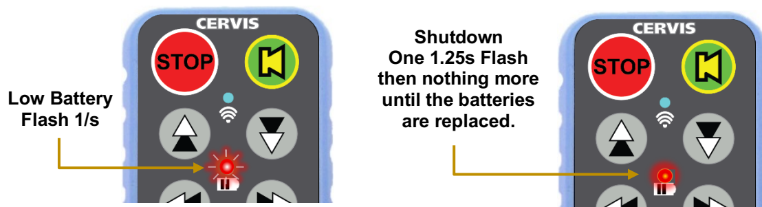
Figure 4. HH2S-9XW10 Remote Low Battery Warning and Auto-Shutdown
