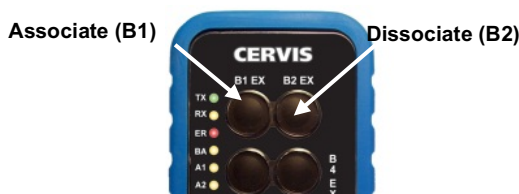
Figure 5. Remote Control Unit to BU-x18XF/BU-xH18XF Associate Example
