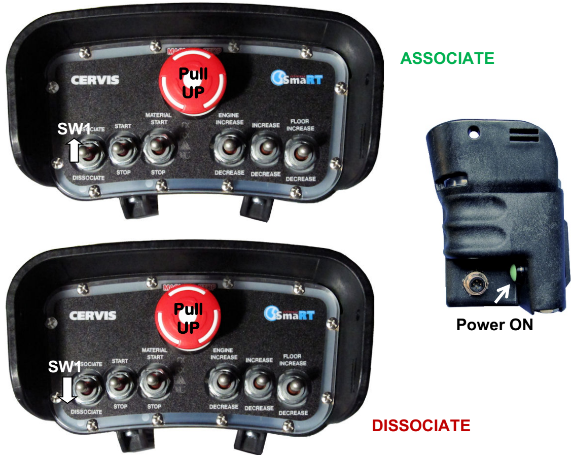
Figure 11. MCB Switch Actuation for Associate and Dissociate
