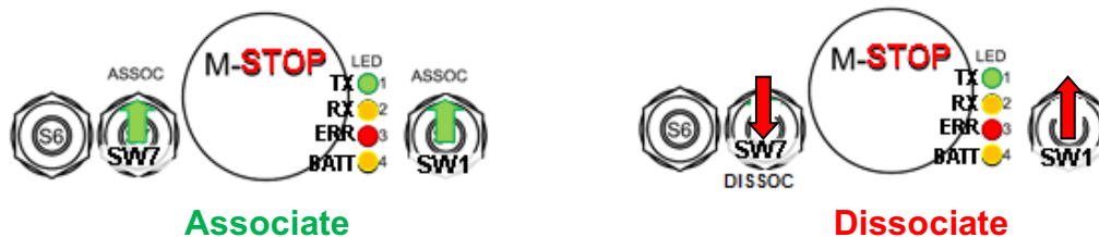
Figure 12. PG Switch Actuation for Associate and Dissociate
