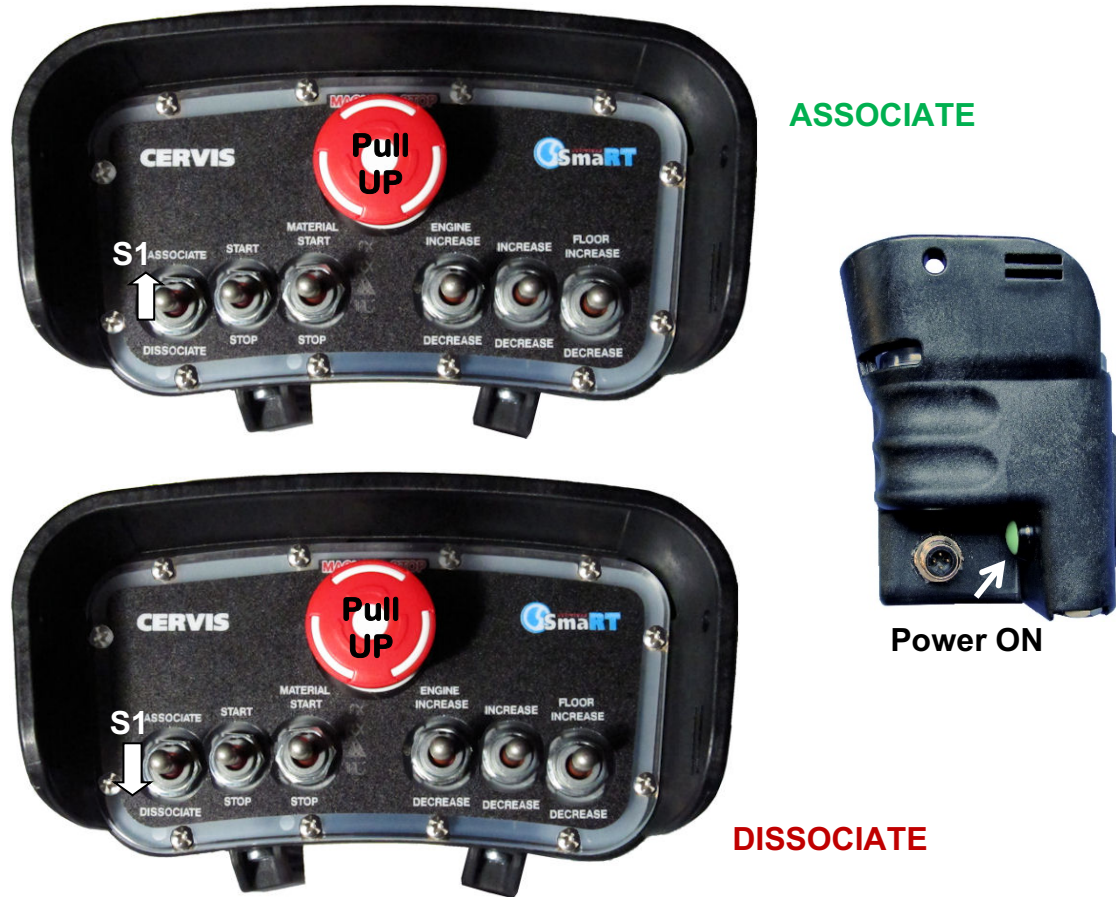
Figure 10. MCB Switch Actuation for Associate and Dissociate
