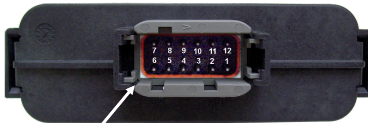
P1 Connector. P1 PIN Numbers are enhanced here for ease of identification.
