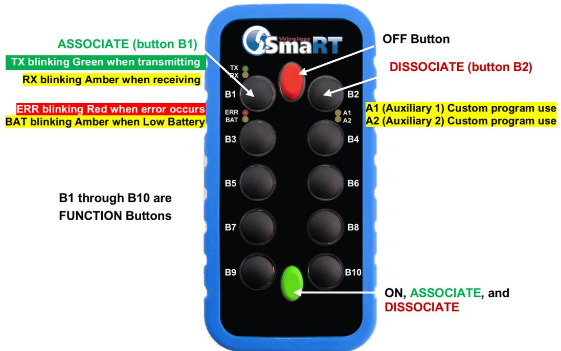
*Figure 6. HH-x10 Front Panel*
