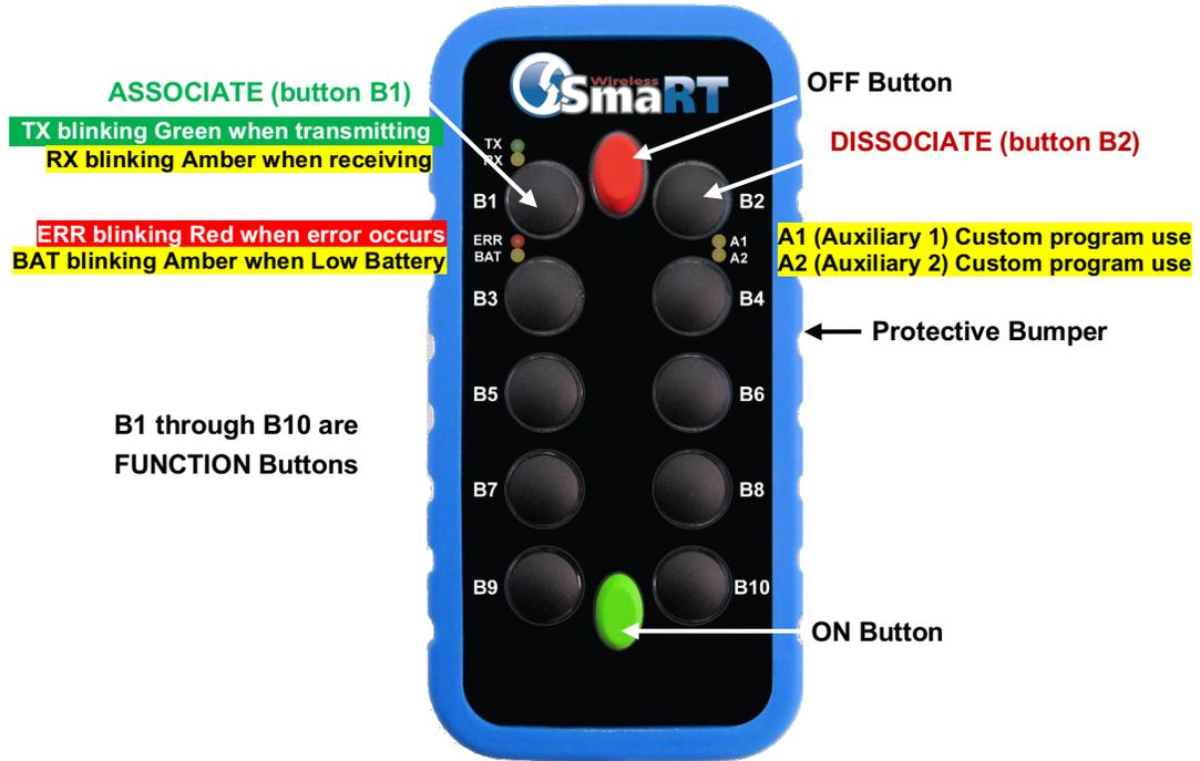
*Figure 2. Standard Ten-Button Example*
