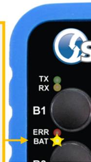
Figure 7. HH-x10 Remote Low Battery Warning and Auto-Shutdown
