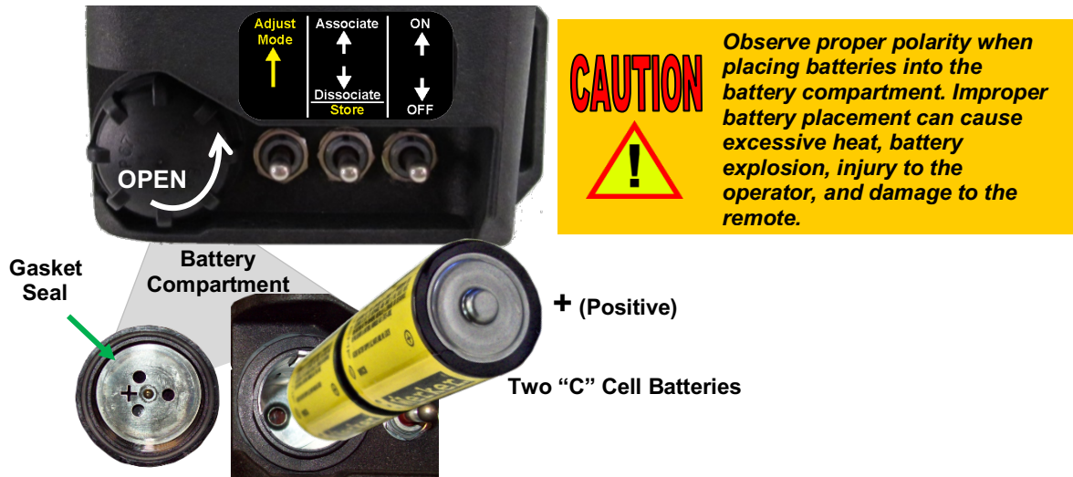
Figure 3. SmaRT Console Box Battery Installation
