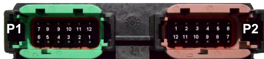
Figure 5. Dual Connectors/Pin Numbers (enhanced)
