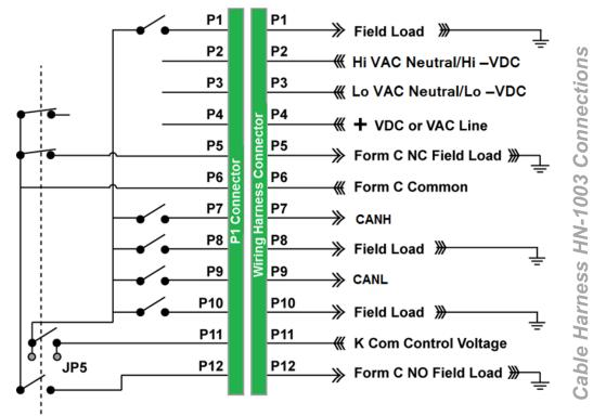
JP5 when installed (factory) isolates Form A relays from the Form C relay.
