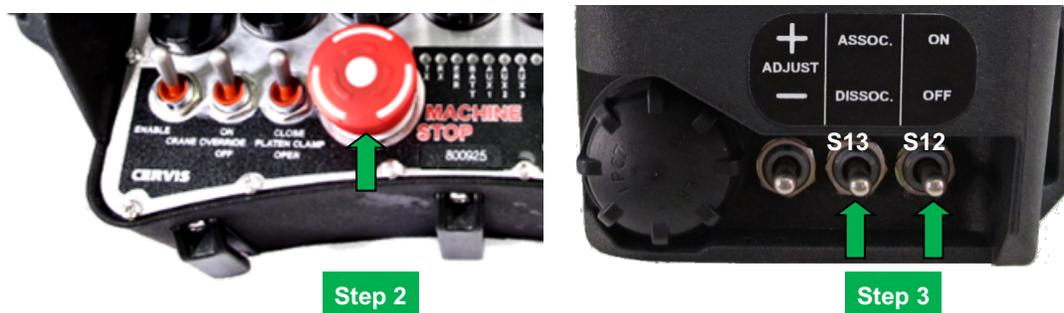
Figure 5. CB-xH Remote to BU-xH20XF Base Unit Associate Example
