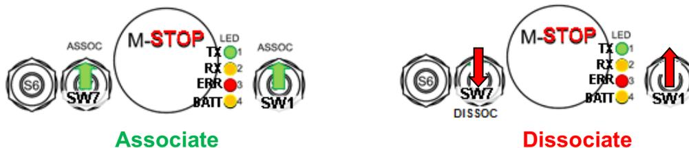
Figure 9. PG Switch Actuation for Associate and Dissociate
