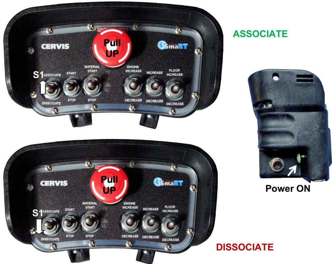
**Figure 8. MCB Switch Actuation for Associate and Dissociate**
