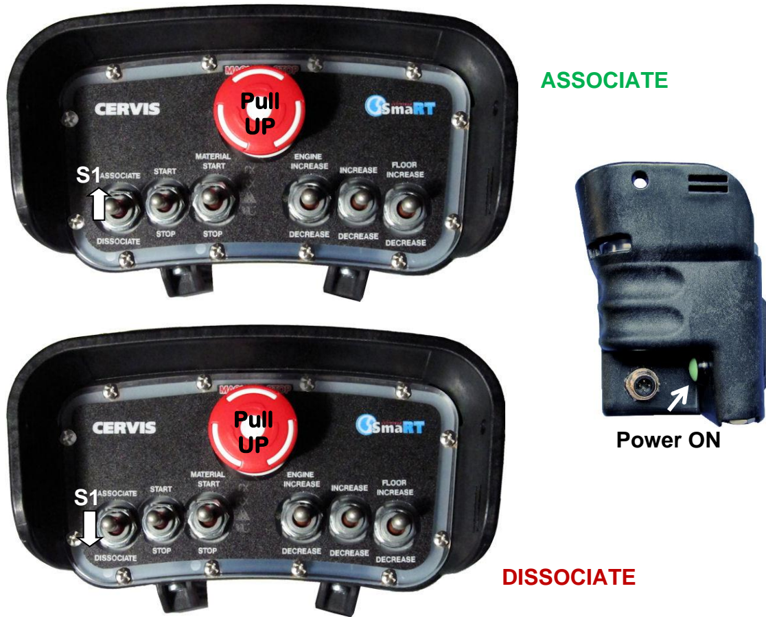
Figure 8. MCB Switch Actuation for Associate and Dissociate
