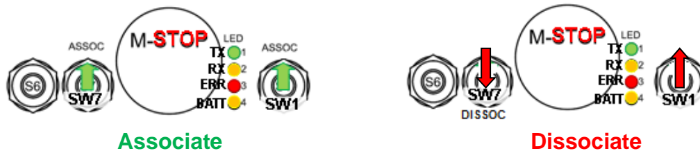
Figure 9. PG Switch Actuation for Associate and Dissociate
