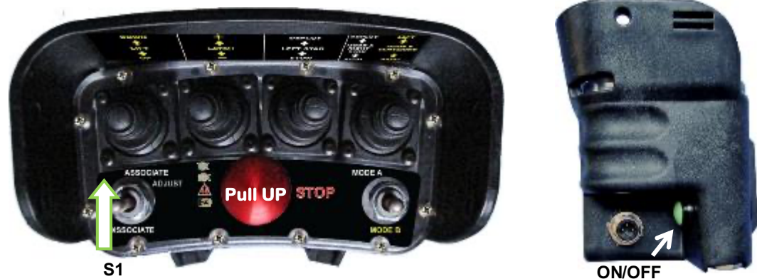
Figure 5. MCB Switch Activation for Associate Mode
