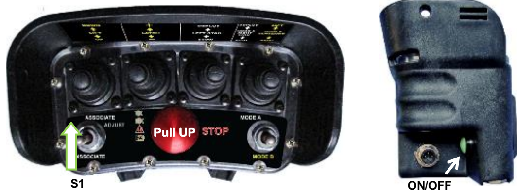
Figure 5. MCB Switch Activation for Associate Mode
