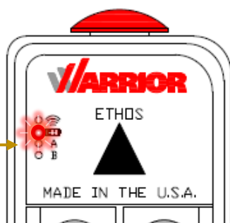
Figure 4. HHMS-9XW08 Remote Low Battery Warning and Auto-Shutdown
