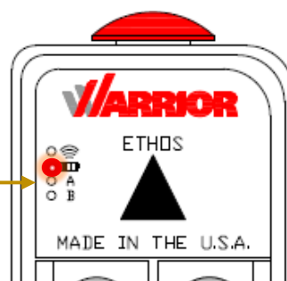
Figure 4. HHMS-9XW08 Remote Low Battery Warning and Auto-Shutdown
